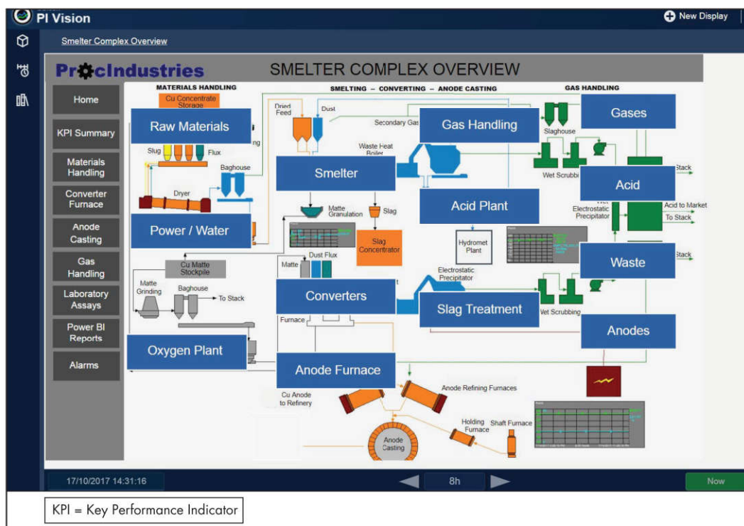
Figure 16 Smelter process model context for data modeling for performance management
