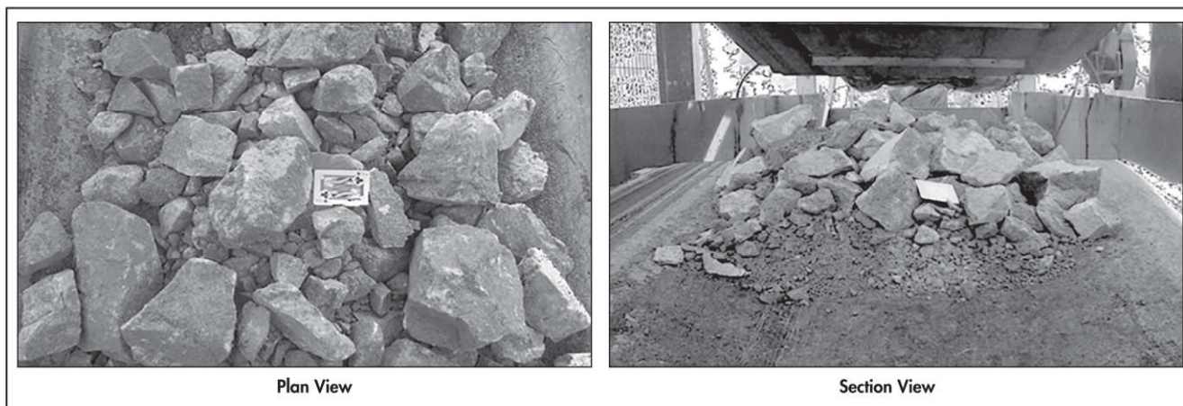
Figure 12 Hidden fines on a conveyor belt
