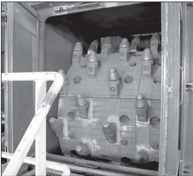
Figure 13 Maintenance access to primary double-roll crusher
