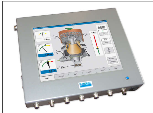
Figure 10 Interface for the ASRi control system
