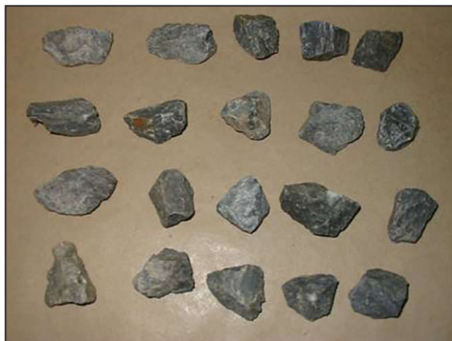
Figure 9 Particles selected for SMC testing from crushed rock
