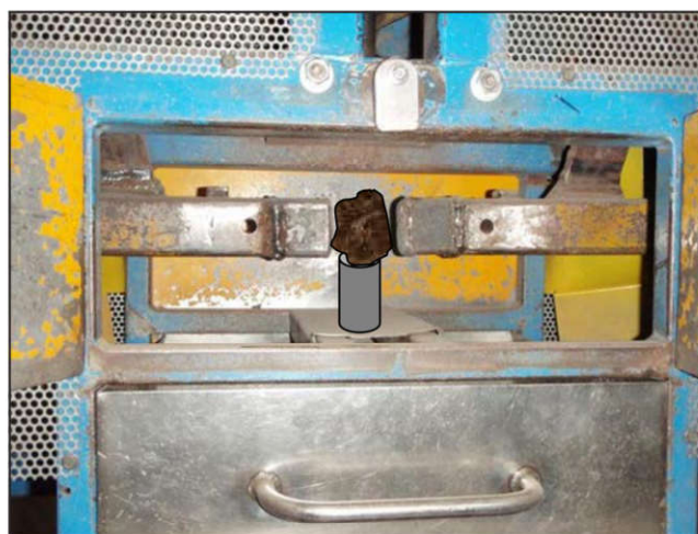
Figure 1 Region where breakage takes place in Bond's crushing work index machine
