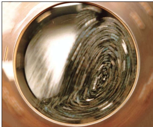
Figure 53 Charge inside a rotating mill
