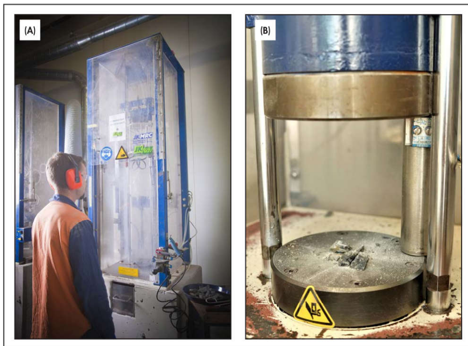
Figure 29 (A) Drop weight test in operation and (B) close-up of impact head and anvil
