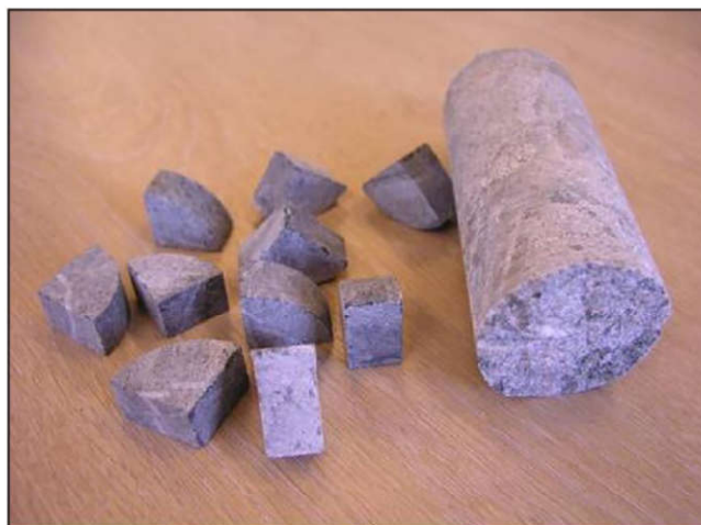
Figure 8 Particles selected for SMC testing from cutting drill core
