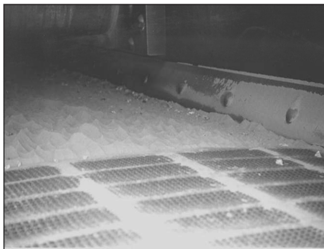
Figure 16 Blinding on a screen deck
