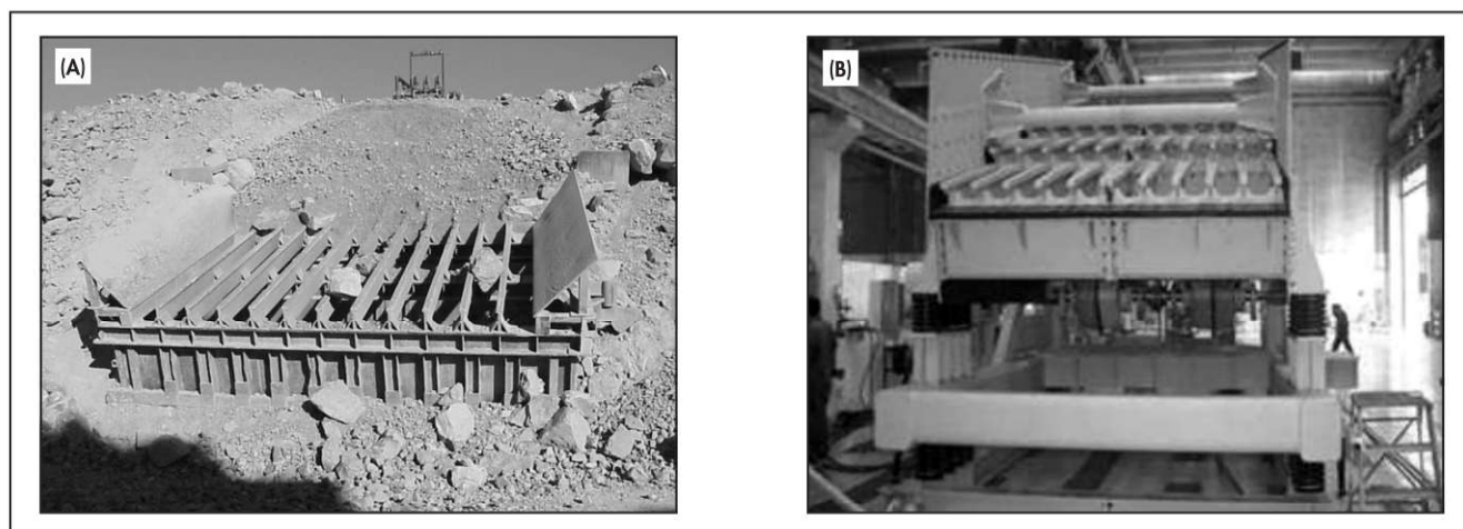
Figure 2 (A) Static grizzly (scalping oversize from a primary jaw crusher feed) and (B) vibrating grizzly screen
