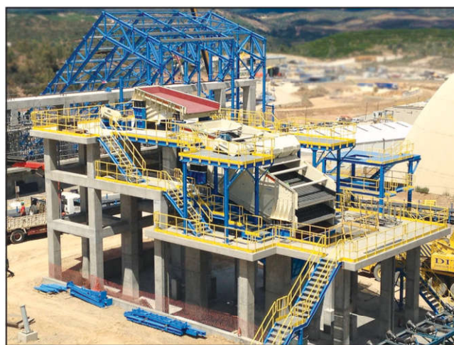
Figure 34 Large screen fed by a divergent vibrating feeder
