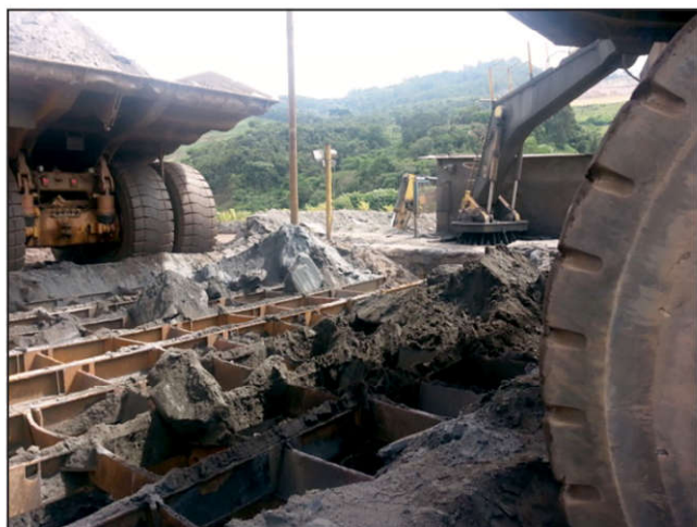
Figure 31 Static grid at primary crushing dump point
