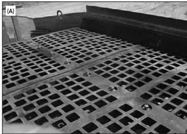
Source: Flintoff and Kuehl 2011 Figure 27 Rubber screen decks
