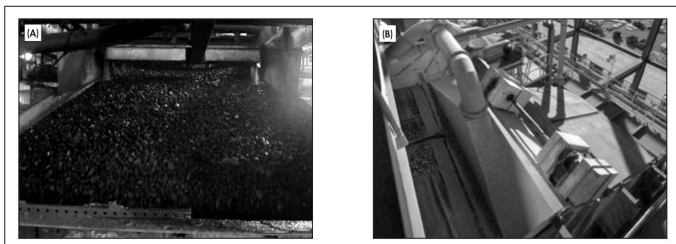
Figure 3 Vibrating screen with a dust collection system
