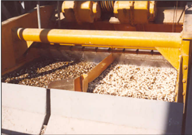
Figure 40 Drain-and-rinse screen with partition wall
