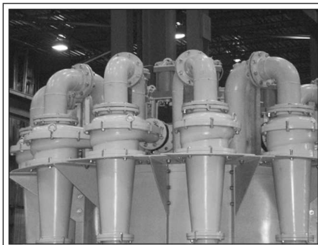
Figure 3 Side and top views of hydrocyclone clusters
