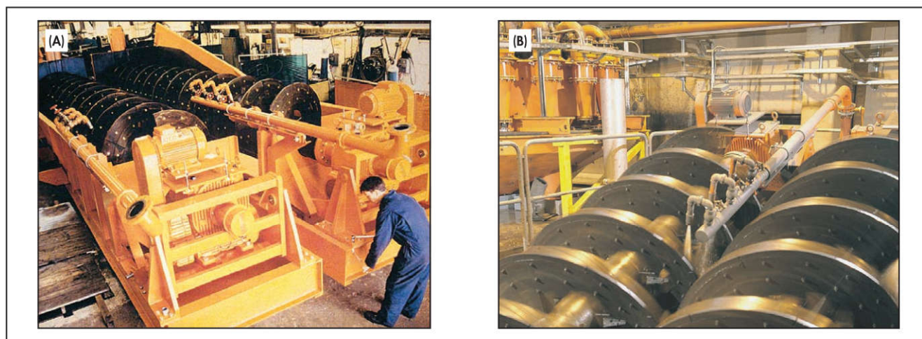
Figure 9 (A) Single- and (B) double-spiral screw classifiers
