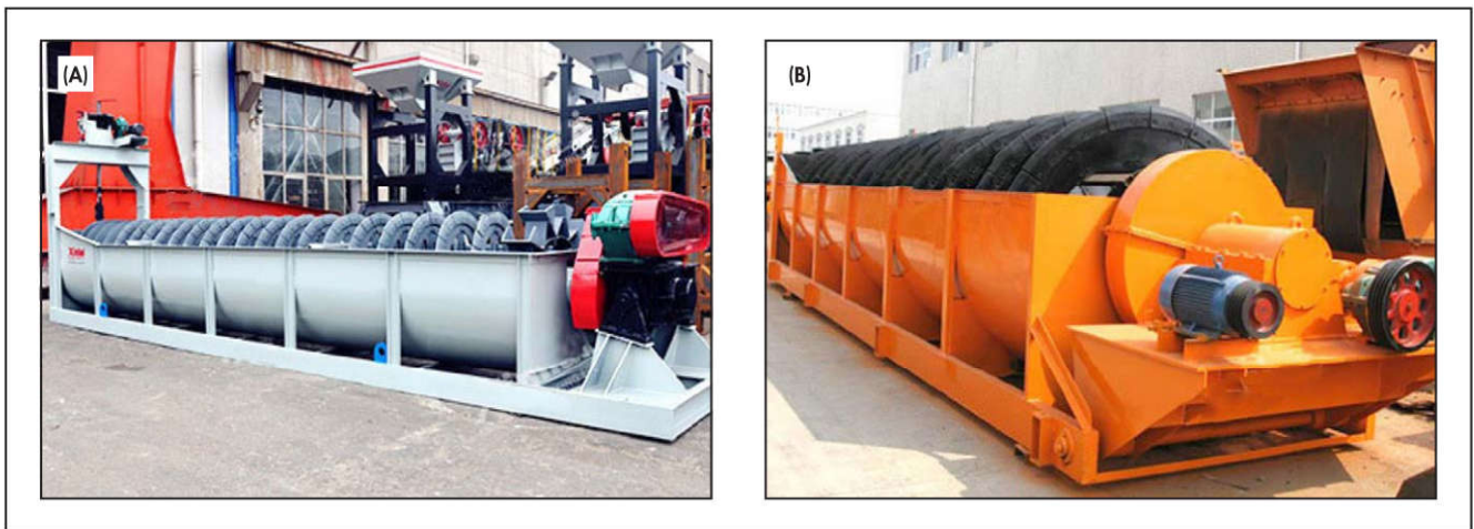
Figure 10 (A) High weir and (B) submerged spiral classifiers
