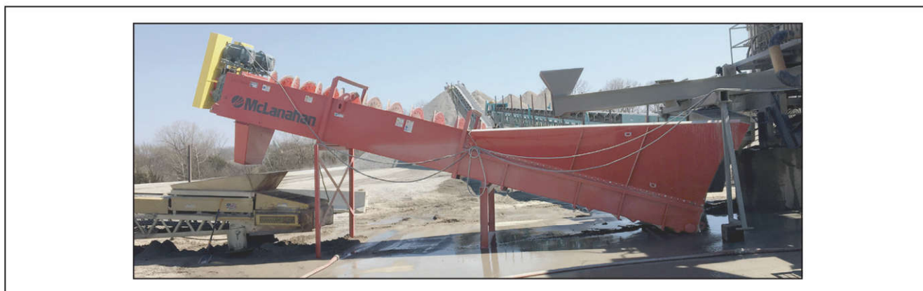
Figure 7 Fine-material screw classifier
