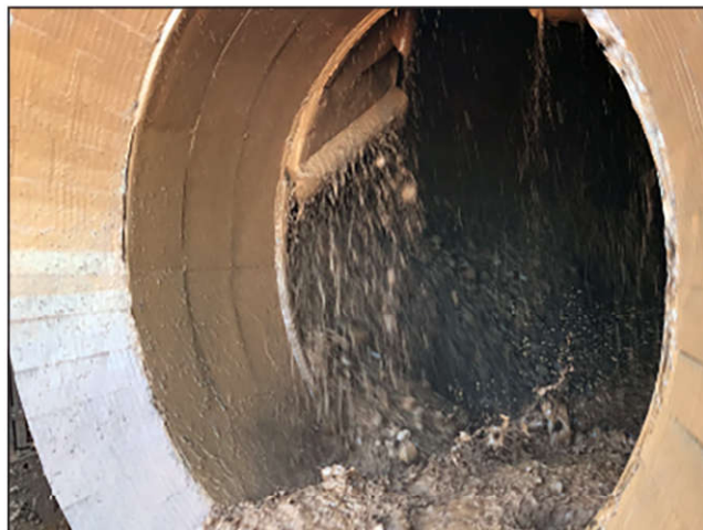
Figure 9 Scrubber internal view with solids pile at dynamic angle of repose
