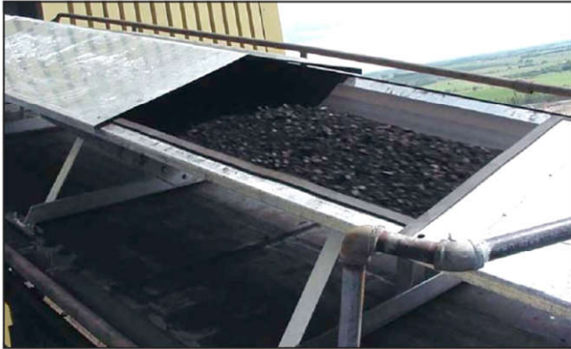
Figure 27 Air-supported conveyor with one cover section removed
