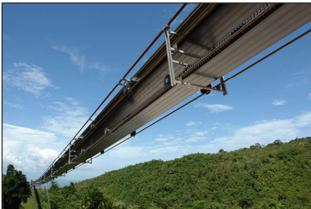
Courtesy of Doppelmayr Transport Technology Figure 29 Section of a large overland RopeCon system
