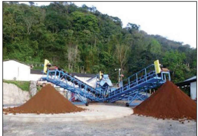
Figure 5 Bulk diversion of nickel laterites via X-ray fluorescence analysis to product stockpile (right) and waste stockpile (left)
