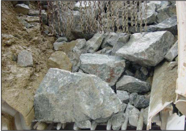
Figure 37 Provisions for impact and/or abrasion resistance in feed and discharge areas are important in primary applications
