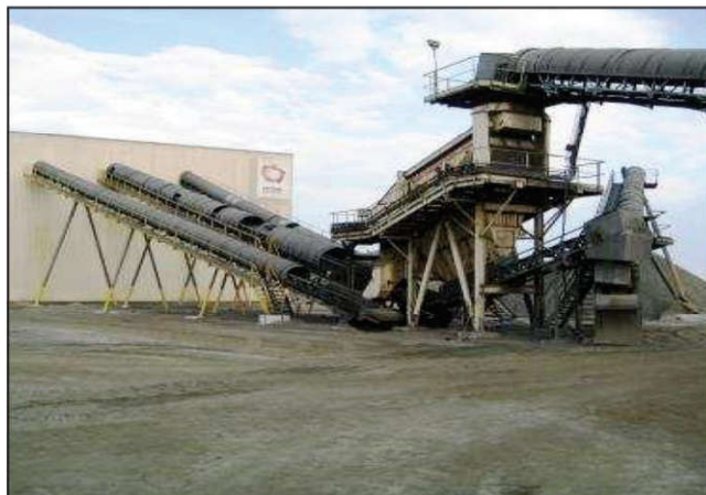
Figure 38 X-ray fluorescence (XRF)-based platinum sorting plant
