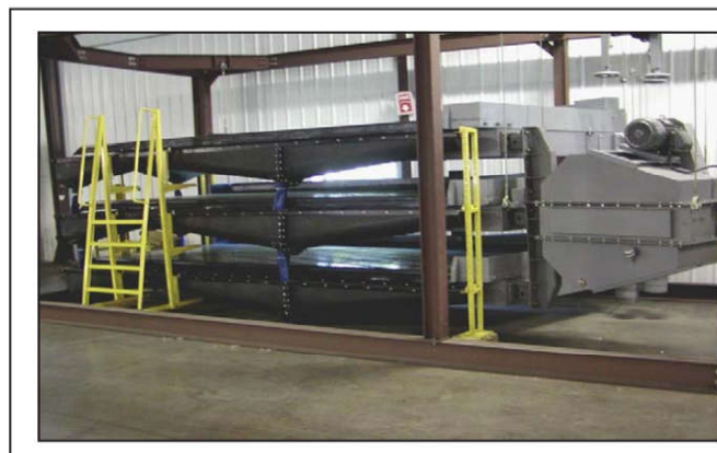
Figure 16 Deister triple-deck tables and slime deck covering
