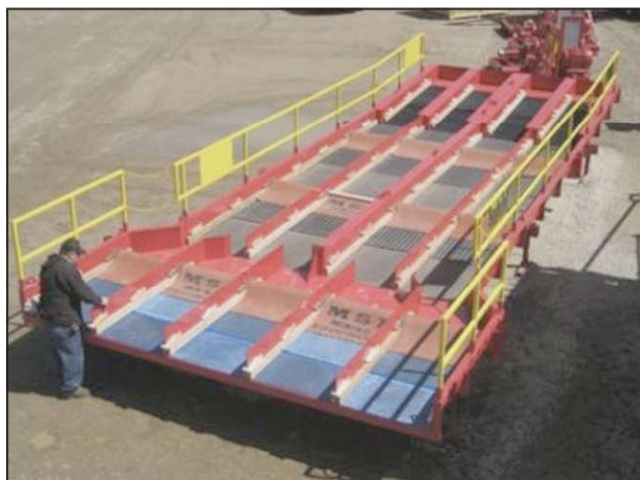
Figure 11 Large sluice box for gold (~5 × 12 m)
