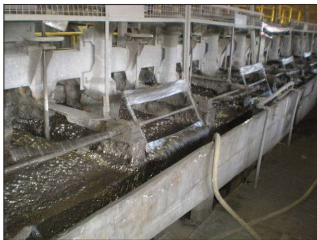
Figure 15 Froth overflow in a cell with a froth paddle
