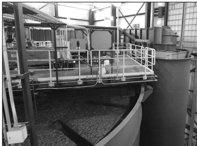
Figure 19 FLSmidth 660-m 3 SuperCell ® machine with radial launders
