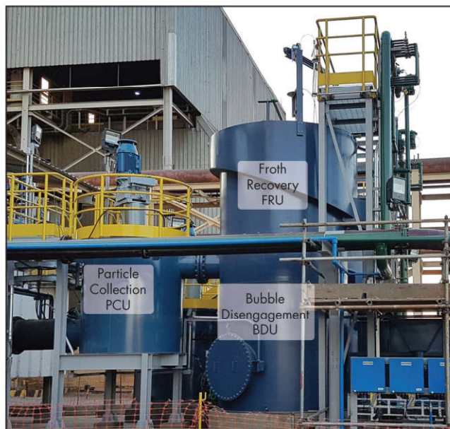
Figure 13 SFR machine, with agitation chamber on the left and separation chamber on the right
