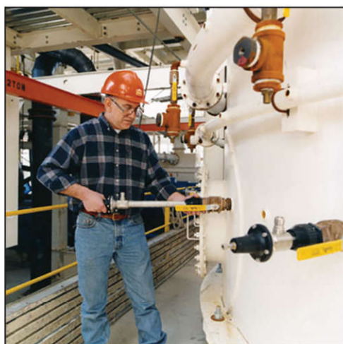
Figure 14 Externally serviceable, self-closing, high-velocity gas sparger
