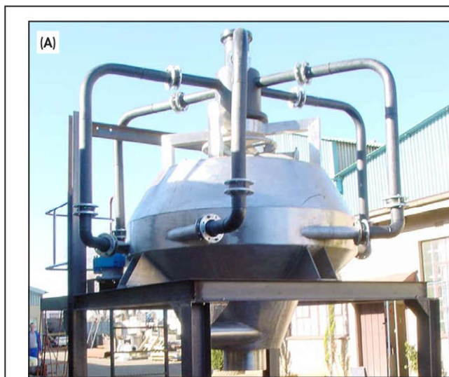
Figure 10 (A) Assembled G-cell and (B) centrifugal flow of pulp
