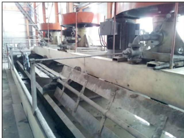
Figure 9 Froth paddles together with trough-style flotation cells (partially empty)
