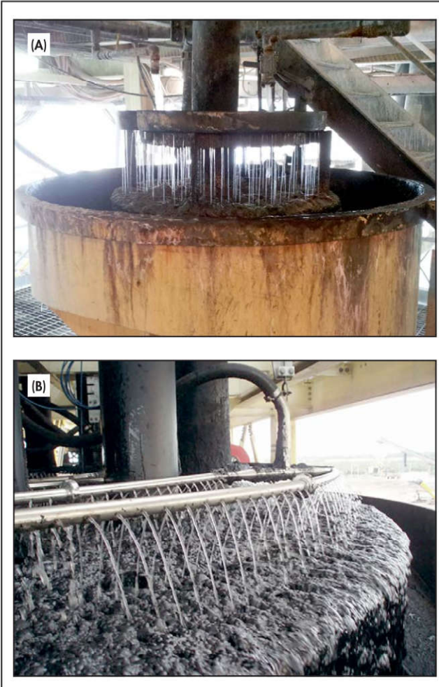
Figure 7 Suspended (A) wash-water trough and (B) wash-water ring providing wash water
