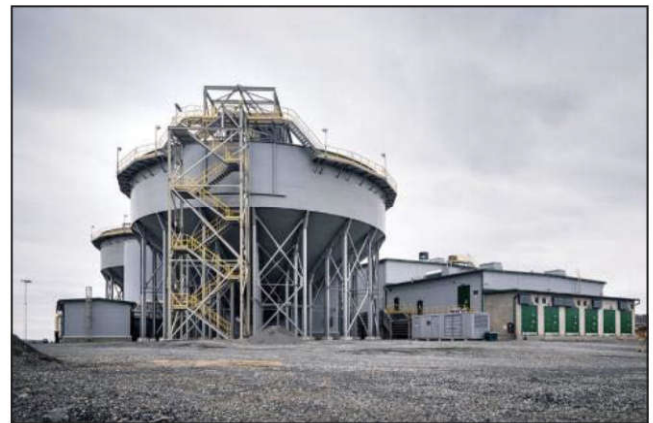
Figure 15 Paste thickener, 30-m diameter with 40-degree floor slope
