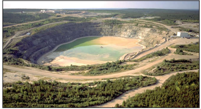
Figure 4 In-pit disposal at Langer Heinrich mine, Africa
