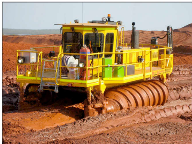
Figure 10 Mechanical drying of tailings
