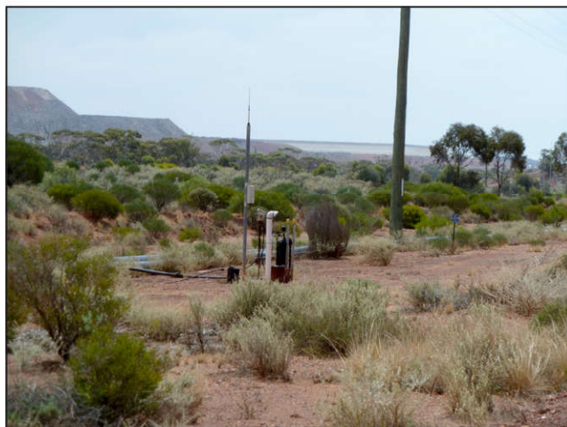
Figure 15 Typical piezometer (fitted with a telemetry system)
