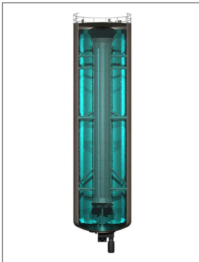
Figure 7 Draft tube reactor with bottom-entry agitator
