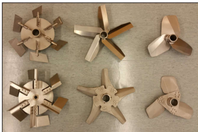
Figure 9 Impellers containing no welded joints and their welded duplicates
