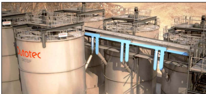
Figure 10 Gravity flow launder connecting reactors in series
