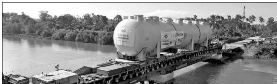
Figure 19 Autoclave vessel transportation for the Pueblo Viejo Project, Dominican Republic
