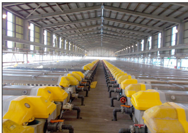
Figure 8 Commercial copper tankhouse with acid mist capture hoods
