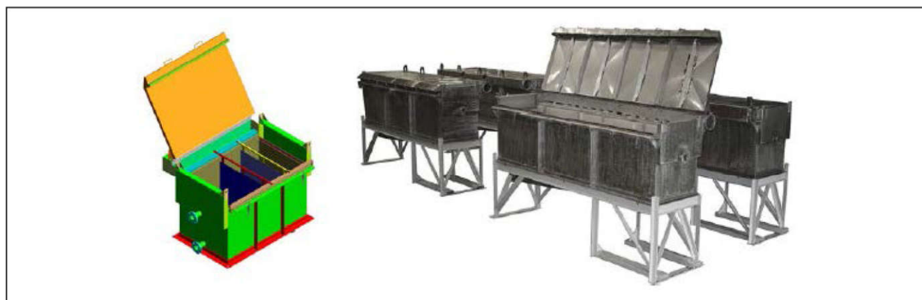
Figure 13 Schematic drawing and photograph of gold electrowinning cells
