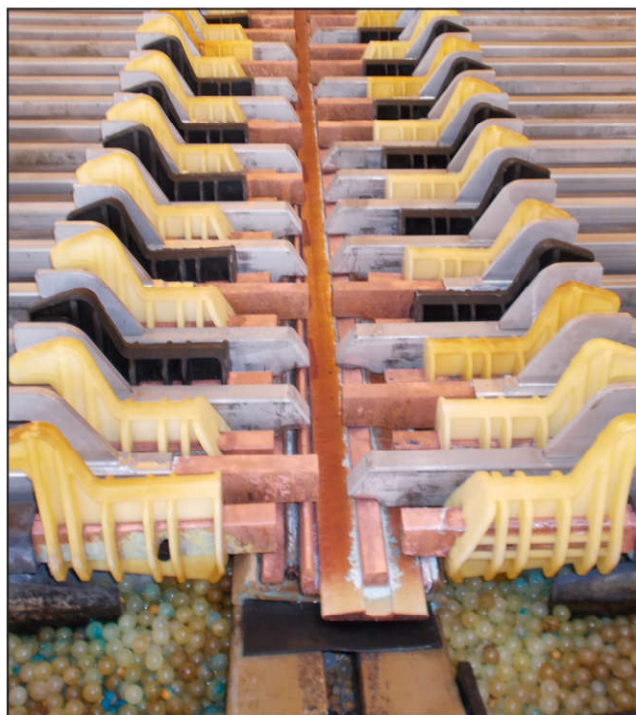
Figure 10 Electrodes resting on a contact system in a copper electrowinning facility
