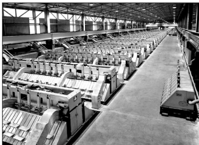
Figure 4 Modern side-by-side 300+ kA cell line in Sunndalsøra, Norway
