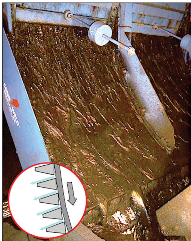
Figure 4 Fine-wire sieve bend
