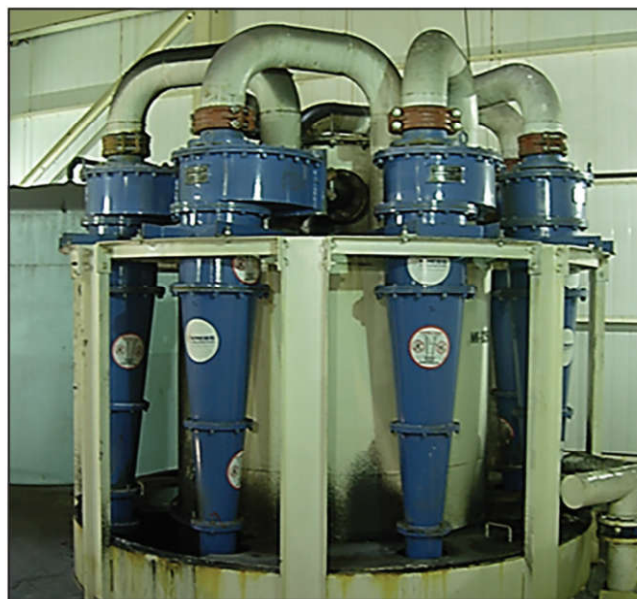
Figure 5 Classifying cyclone bank
