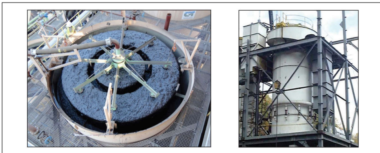
Figure 13 Installation of column flotation cells
