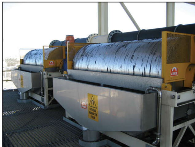
Figure 8 Drum-style magnetic separators
