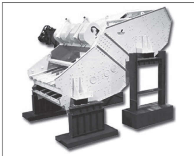
Figure 3 Multi-slope banana screen
