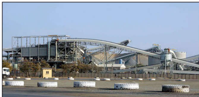
Figure 14 Preconcentration of low-grade nickel ores at the Tati nickel mine
