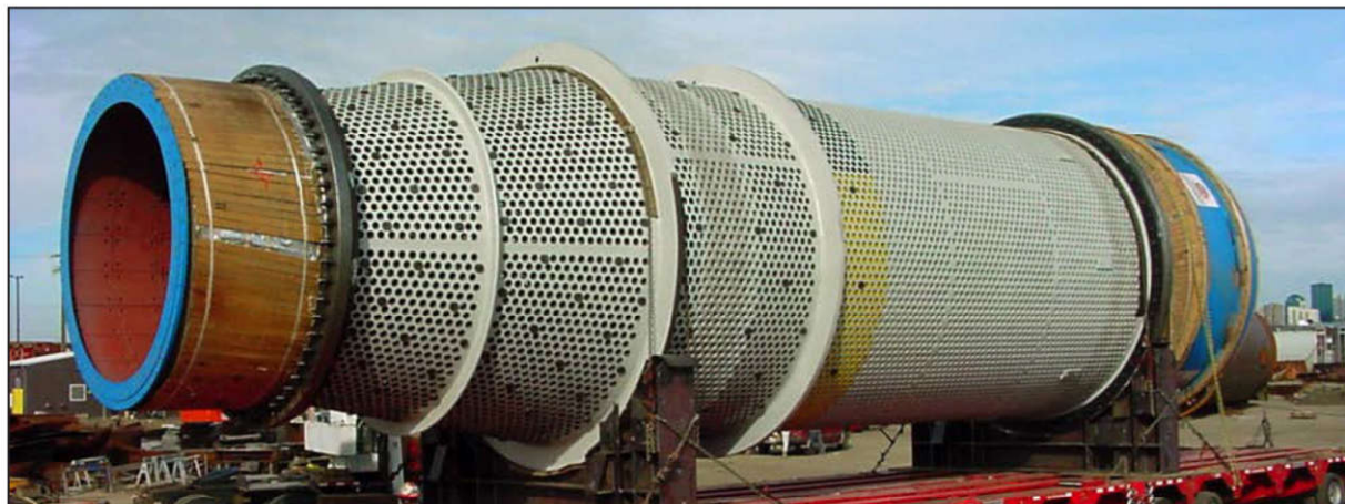
Figure 7 ThyssenKrupp rotary breaker for a typical slurry preparation system
