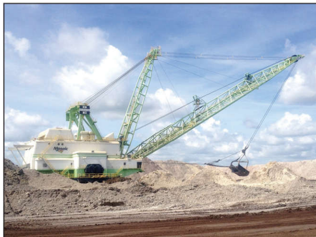
Figure 3 Surface mining of phosphate rock with dragline in Florida, United States
